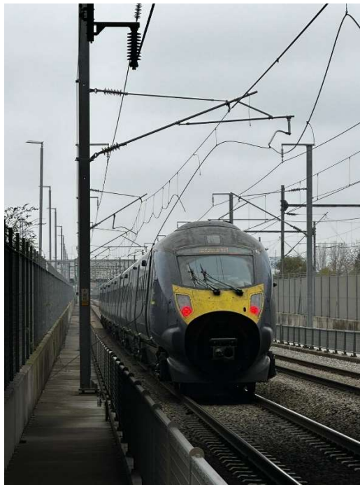
FIGURE 4 -STRANDED TRAIN BELOW OHLE DEWIREMENT
